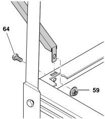
12. Tighten all hexagon head screws and flange nuts of the saw's stand.
